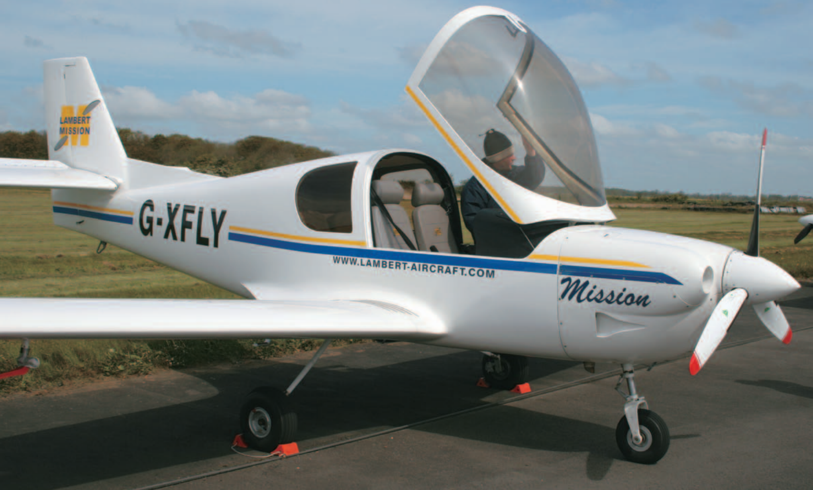
The large forward hinging canopy allows good cockpit access. An inflatable seal will add to passenger comfort on production kits.
