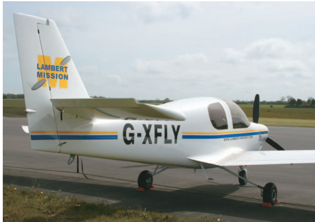
The fuselage step greatly aids access to the wing-walk. The less energetic would also find a grab handle useful. Note also Cessna style gear legs, which will be uprated in production aircraft.
